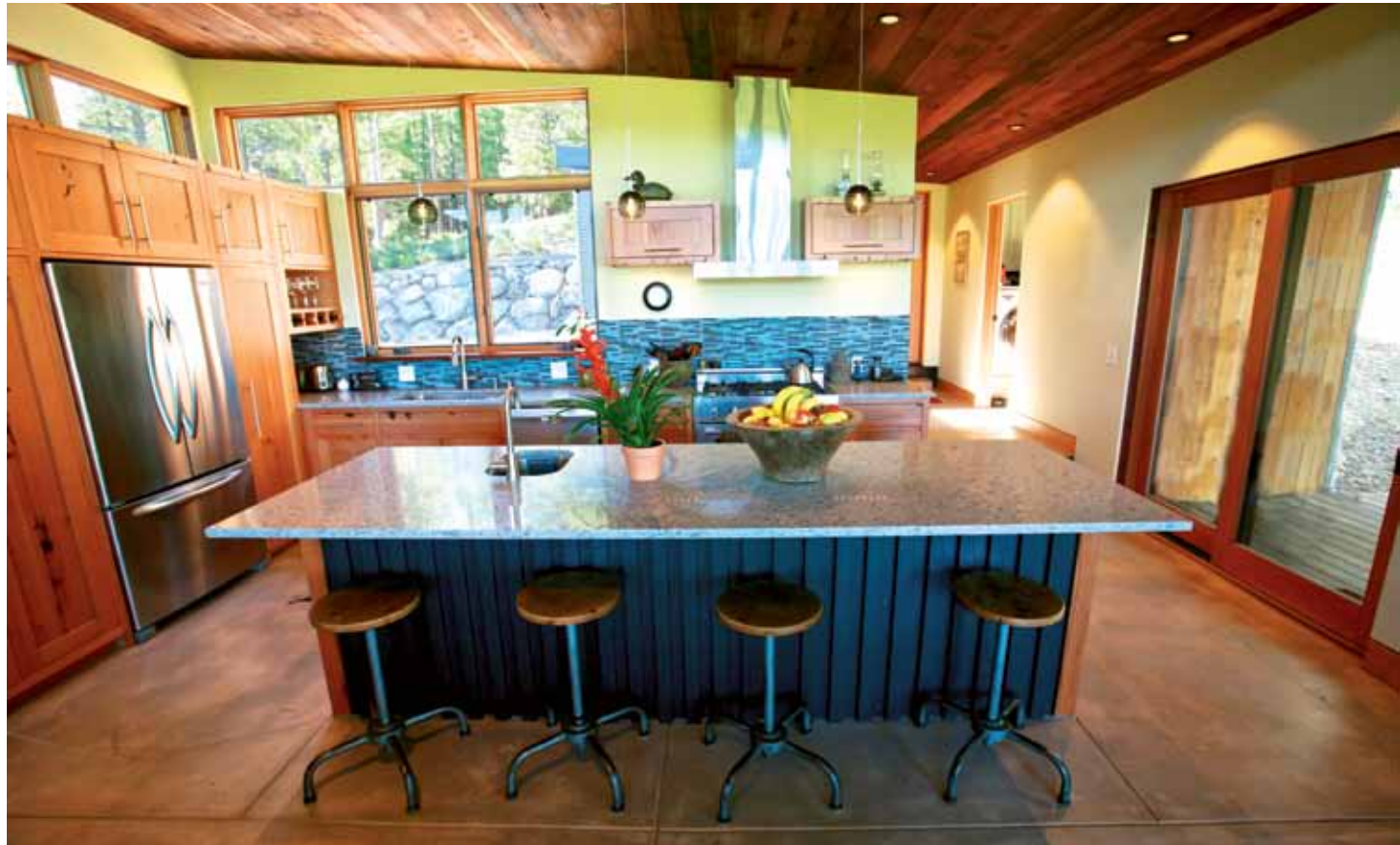
The ultra efficient building envelope allows the winter sun to penetrate deep into the interior, warming the concrete floors and augmenting the active radiant heat, while the large porch overhang keeps summer sun far away from the south windows
